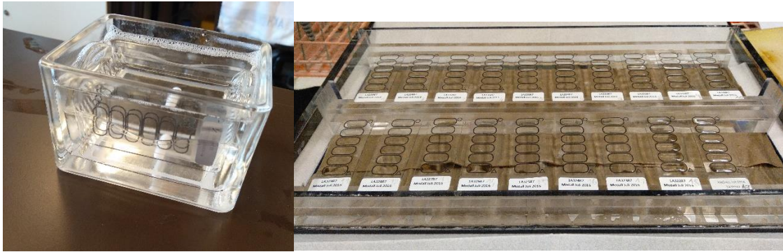
Figure 1. Chips into washing buffer, on magnetic stirrer / Figure 2. Each chip comprises 6 arrays containing serum or sample diluent/calibrator.
