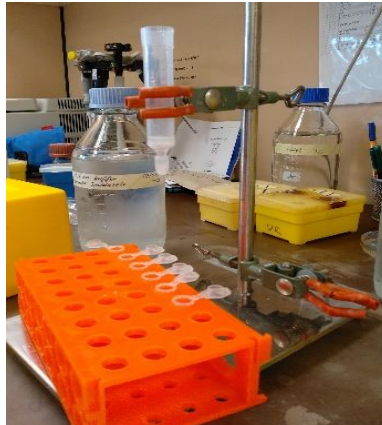
Figure 8. Purification of recombinant protein on Ni-NTA resin in a column.
